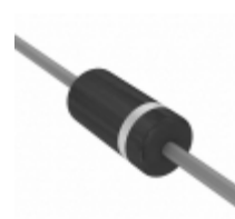
P6KE15A-E3/54 Vishay Semiconductor Diodes Division TVS DIODE 12.8VWM 21.2VC DO204AC
