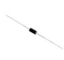
P6KE15A Littelfuse Inc. TVS DIODE 12.8VWM 21.2VC DO204AC
