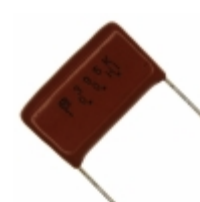
ECQ-E1395JFW Panasonic Electronic Components CAP FILM 3.9UF 5% 100VDC RADIAL
