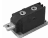
VSKT170-16 Vishay Semiconductor Diodes Division SCR DBL HISCR 1600V 170A MAGNPAK
