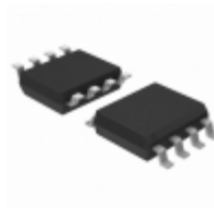
ATECC108-SSH CZ-B Microchip Technology ECC 8KB 8-SOIC SINGLE WIRE BULK
