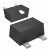
DTC015EUBTL Rohm Semiconductor TRANS PREBIAS NPN 50V 0.2W UMT3F
