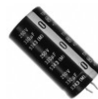
ECE-S2EG331N Panasonic Electronic Components CAP ALUM 330UF 20% 250V SNAP
