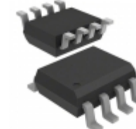
AD8041AR-REEL Analog Devices Inc. IC OPAMP VFB 170MHZ RRO 8SOIC
