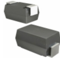
3SMAJ5945B-TP Micro Commercial Co DIODE ZENER 68V 3W DO214AC
