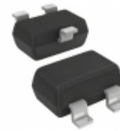
CMST5087 BK Central Semiconductor Corp TRANS PNP 50V 0.05A SOT323
