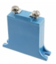
B32K385 EPCOS (TDK) VARISTOR 620V 25KA CHASSIS
