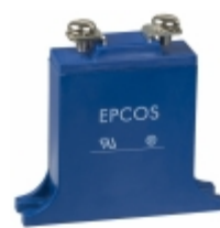
B32K130 EPCOS (TDK) VARISTOR 205V 25KA CHASSIS
