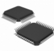
STM32F042C4T6 STMicroelectronics IC MCU 32BIT 16KB FLASH 48LQFP
