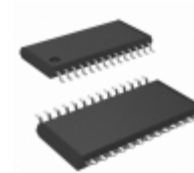
AD9762ARUZ Analog Devices Inc. IC DAC 12BIT 125MSPS 28-TSSOP
