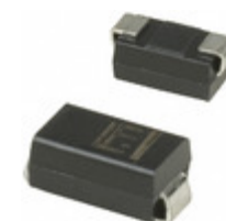
P4SMA30A Littelfuse Inc. TVS DIODE 25.6VWM 41.4VC SMD
