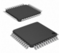
PIC24FJ64GA004-E/PT Micrel / Microchip Technology IC MCU 16BIT 64KB FLASH 44TQFP
