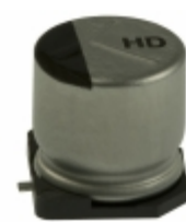
EEE-HD1H3R3R Panasonic Electronic Components CAP ALUM 3.3UF 20% 50V SMD
