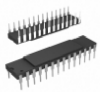
STK12C68-C35I Cypress Semiconductor Corp IC NVSRAM 64KBIT 35NS 28CDIP
