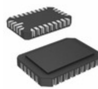
STK12C68-L45I Cypress Semiconductor Corp IC NVSRAM 64KBIT 45NS 28LCC
