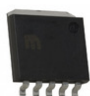
MIC37301-1.5BR Microchip Technology IC REG LDO 1.5V 3A SPAK-5
