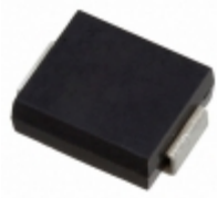
MASMCJLCE7.5A Microsemi Corporation TVS DIODE 7.5VWM 12.9VC DO215AB
