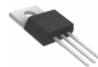
KSD401FYTU AMI Semiconductor / ON Semiconductor TRANS NPN 150V 2A TO-220
