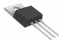
KSD4010 AMI Semiconductor / ON Semiconductor TRANS NPN 150V 2A TO-220
