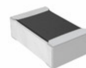
PCF0805-12-200KBT1 TT Electronics/Welwyn RES SMD 200K OHM 0.1% 1/10W 0805
