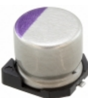
4SVPC330MY Panasonic Electronic Components CAP ALUM POLY 330UF 20% 4V SMD
