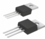
TIP125-BP Micro Commercial Co TRANS PNP DARL 60V 5A TO-220
