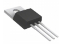
TIP125 Fairchild/ON Semiconductor TRANS PNP DARL 60V 5A TO-220
