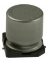
EEE-FK2A470AQ Panasonic Electronic Components CAP ALUM 47UF 20% 100V SMD
