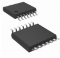
ADA4096-4ARUZ Analog Devices Inc. IC OPAMP GP 786KHZ RRO 14TSSOP
