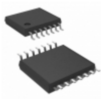
ADA4096-4ARUZ-RL Analog Devices Inc. IC OPAMP GP 786KHZ RRO 14TSSOP
