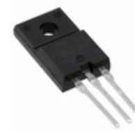
FMKS-2052 Sanken DIODE FAST REC 200V 5A TO-220FP
