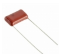
ECQ-E6563KF3 Panasonic Electronic Components CAP FILM 0.056UF 10% 630VDC RAD
