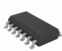
MCP4251-104E/SL Microchip Technology IC DGTL POT 100K 2CH 14SOIC
