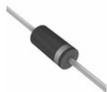
BZW06-20B B0G TSC (Taiwan Semiconductor) TVS DIODE 20.5V 42.8V DO204AC
