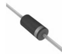
BZW06-20B R0G TSC (Taiwan Semiconductor) TVS DIODE 20.5V 42.8V DO204AC
