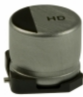
EEV-HD1V220P Panasonic Electronic Components CAP ALUM 22UF 20% 35V SMD
