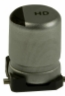
EEV-HD1HR47R Panasonic Electronic Components CAP ALUM 0.47UF 20% 50V SMD
