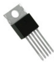
MCP1827-3302E/AT Microchip Technology IC REG LDO 3.3V 1.5A TO220-5
