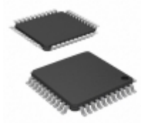
PIC18F43K22T-I/PT Microchip Technology IC MCU 8BIT 8KB FLASH 44TQFP
