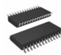
PIC16F18854-I/SO Microchip Technology IC MCU 8BIT 7KB FLASH 28SOIC
