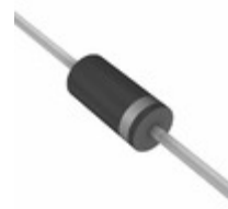
BZW06-48 B0G TSC (Taiwan Semiconductor) TVS DIODE 47.8V 100V DO204AC
