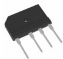
TS40P07G C2G TSC (Taiwan Semiconductor) BRIDGE RECT 1PHASE 1KV 40A TS-6P
