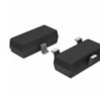
TS4061BILT-1.225 STMicroelectronics IC VREF SHUNT 1.225V SOT23-3
