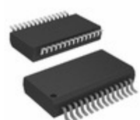
PIC24FJ128GA702-I/SS Microchip Technology IC MCU 16-BIT 128KB FLASH 28SSOP
