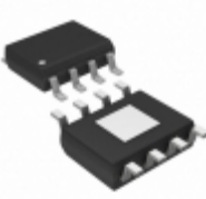
SC4215ASTRT Semtech Corporation IC REG LDO FIX/ADJ 2A 8SOIC
