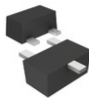
DSC9F0100L Panasonic Electronic Components RF TRANS NPN 10V 1.9GHZ SSMINI3
