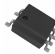
ACPL-M61T-500 Broadcom Limited OPTOISO 4KV OPN COLLECTOR 5SO
