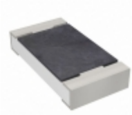
RC1206JR-07240RL Yageo RES SMD 240 OHM 5% 1/4W 1206
