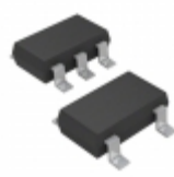
ADP1712AUJZ-1.8-R7 Analog Devices Inc. IC REG LDO 1.8V 0.3A TSOT23-5
