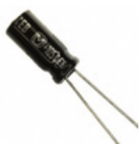
EEU-EB1H1R0S Panasonic Electronic Components CAP ALUM 1UF 20% 50V RADIAL
