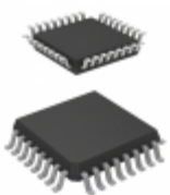
MC68HC908RF2MFA NXP USA Inc. IC MCU 8BIT 2KB FLASH 32LQFP
