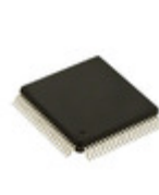
MC68HC912B32CFU8 NXP USA Inc. IC MCU 16BIT 32KB FLASH 80QFP
