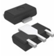
AN78L18ME1 Panasonic Electronic Components IC REG LDO 18V 0.1A 3HSIP
