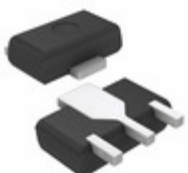
AN78L24ME1 Panasonic Electronic Components IC REG LDO 24V 0.1A 3HSIP
