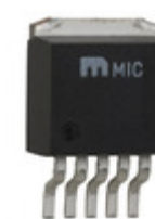
MIC29301-3.3WU-TR Microchip Technology IC REG LDO 3.3V 3A TO263-5
