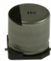
EEE-HC1E331P Panasonic Electronic Components CAP ALUM 330UF 20% 25V SMD
