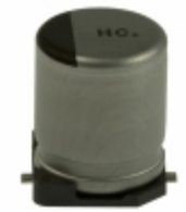
EEE-HC1E101P Panasonic Electronic Components CAP ALUM 100UF 20% 25V SMD
