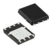
SI7772DP-T1-GE3 Electro-Films (EFI) / Vishay MOSFET N-CH 30V 35.6A PPAK SO-8
