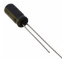
EEU-FC1V221B Panasonic Electronic Components CAP ALUM 220UF 20% 35V RADIAL
