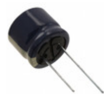
EEU-FC1V182SB Panasonic Electronic Components CAP ALUM 1800UF 20% 35V RADIAL
