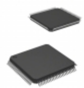
ISPLSI 1024EA-100LT100 Lattice Semiconductor Corporation IC CPLD 64MC 10NS 100TQFP
