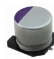
20SVPS47M Panasonic Electronic Components CAP ALUM POLY 47UF 20% 20V SMD
