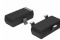
DSA2G01B0L Panasonic Electronic Components TRANS PNP 20V 0.03A MINI3
